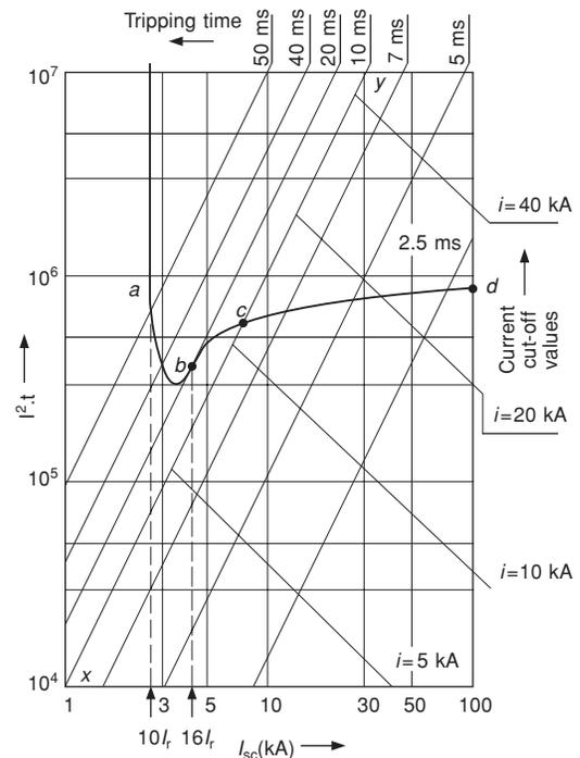
Note : Below the tripping time curve x–y of 10 ms is the current limiting area.
