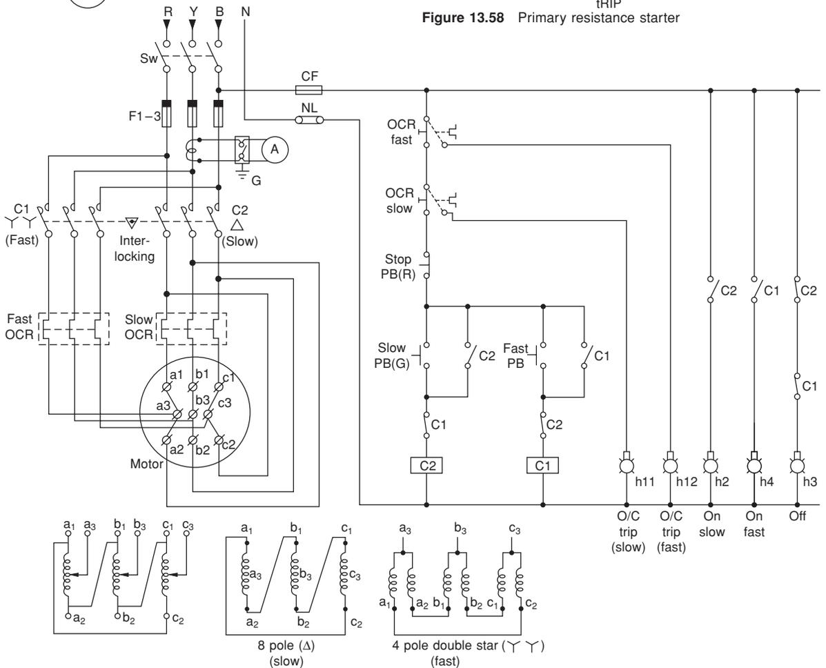
Figure 13.59 Dual-speed starter
