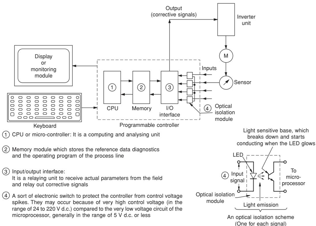
**Figure 13.12** A simple representation of a programmable controller
