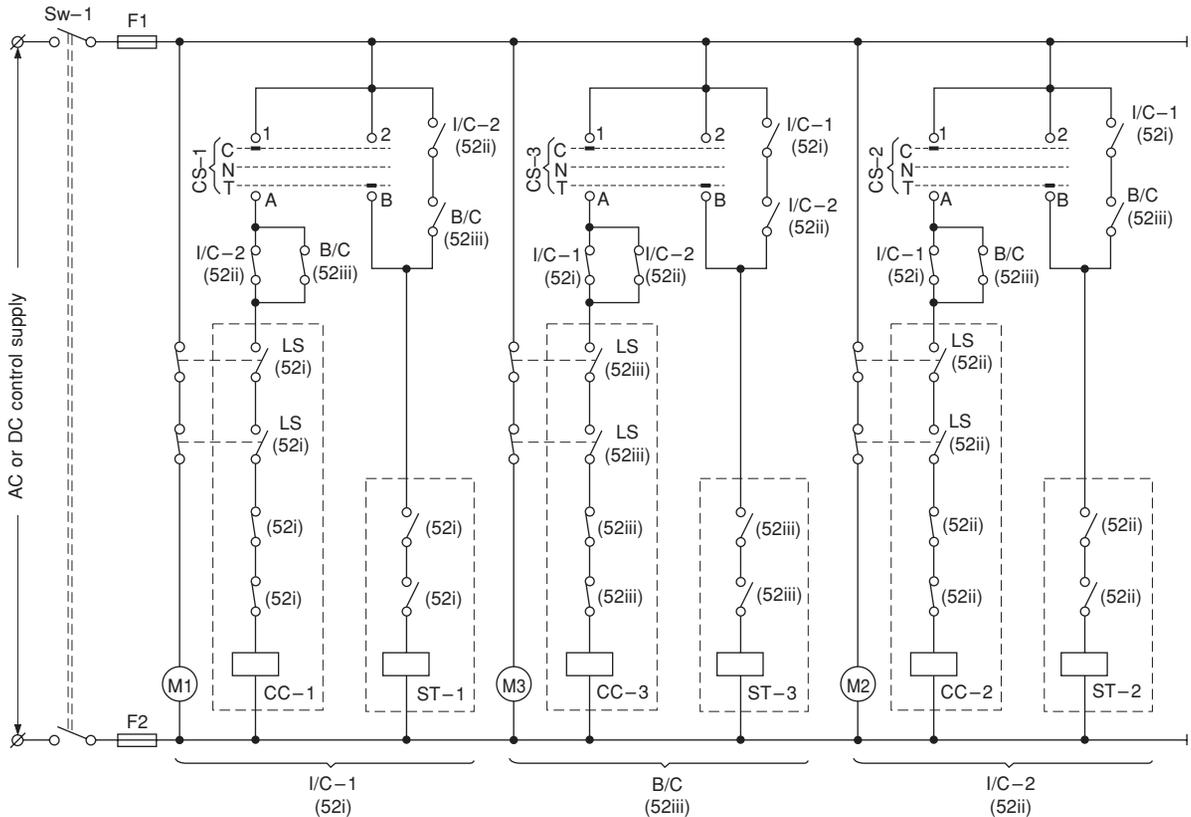
**Figure 13.46** Control scheme for two electrically operated breakers, a bus coupler and two sources of supplies
