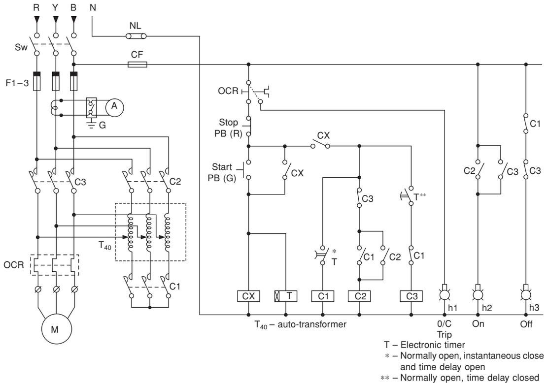
Figure 13.57(b) Auto-transformer starter using electronic timer
