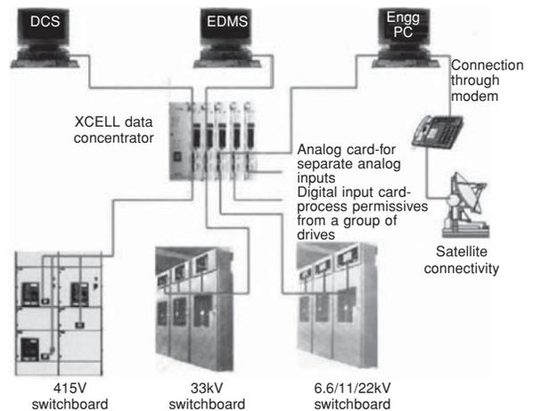
**Figure 13.9(c)** Application of intelligent switchboards for remote monitoring and control for total power automation (Courtesy: Larsen & Toubro)
