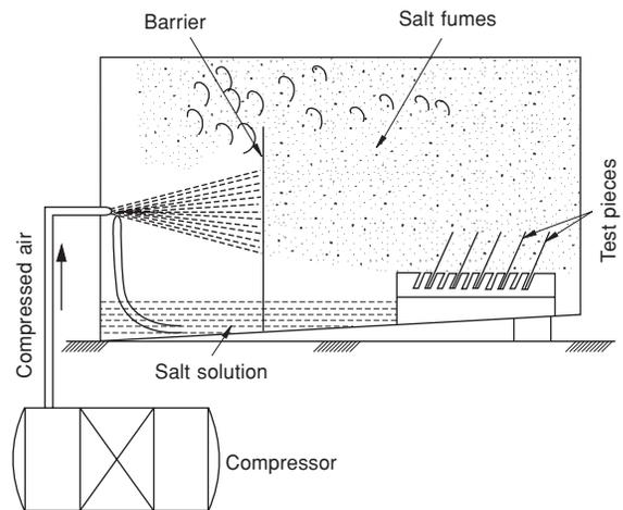
Figure A13.9 Salt spray chamber
