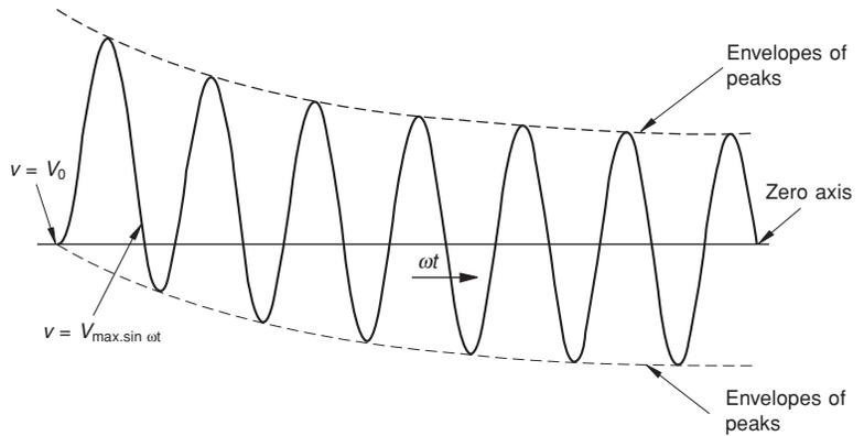
**Figure 13.25** An asymmetrical waveform
