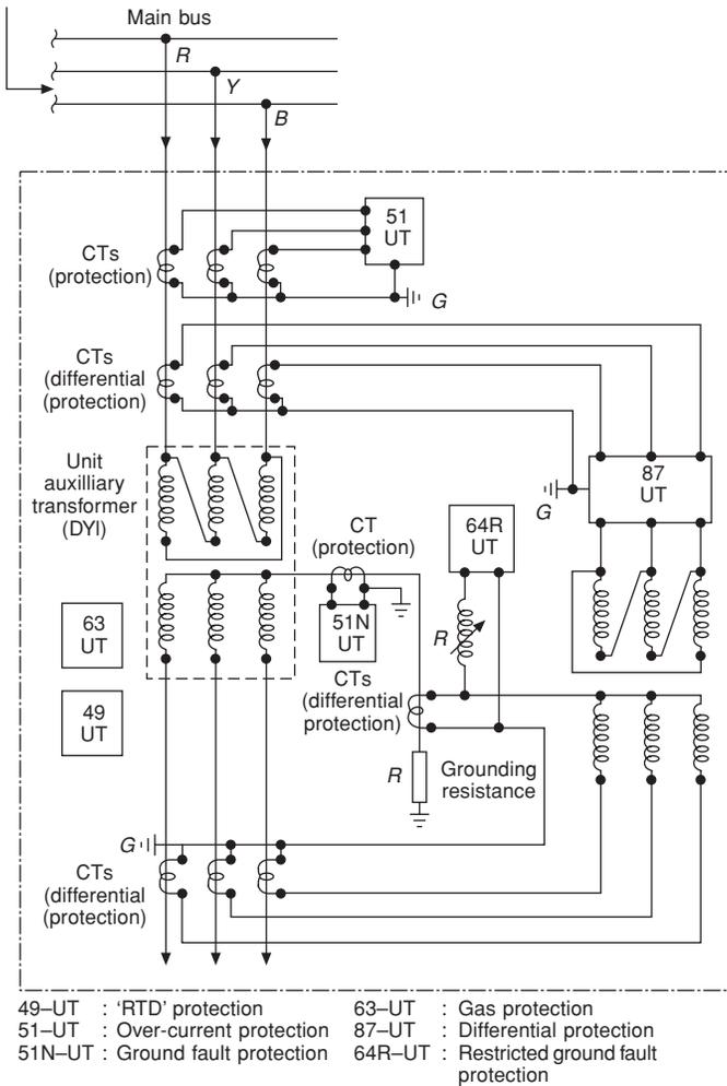
**Figure 13.47(a)** Protection scheme for a unit auxiliary transformer (UAT)
