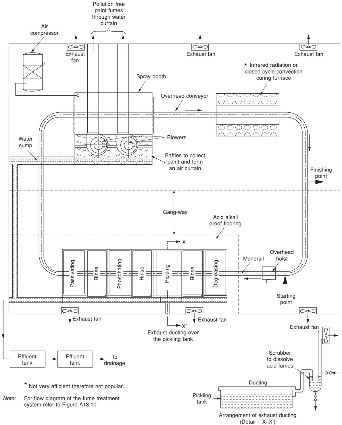
**Figure A13.1** A liquid painting system illustrating typical layout of a medium-sized paint shop showing a seven-tank pre-treatment process
