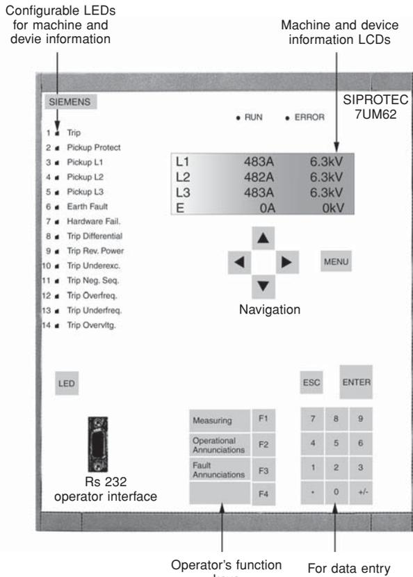
Front view of a multifunction generator, motor and transformer protection relay (Courtesy: Siemens)
