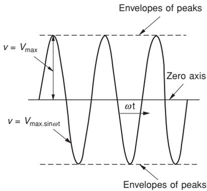
**Figure 13.24** A symmetrical waveform
