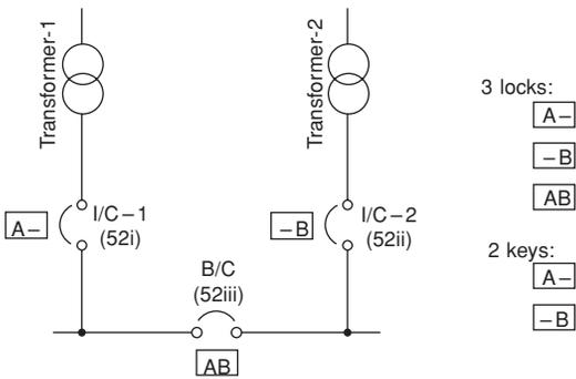
**Figure 13.40** Two sources of supply and a bus coupler
