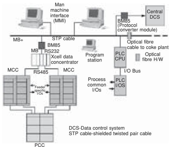
**Figure 13.9(b)** Typical layout of a switch room with remote control station at Tata Steel (Courtesy: Larsen & Toubro)
