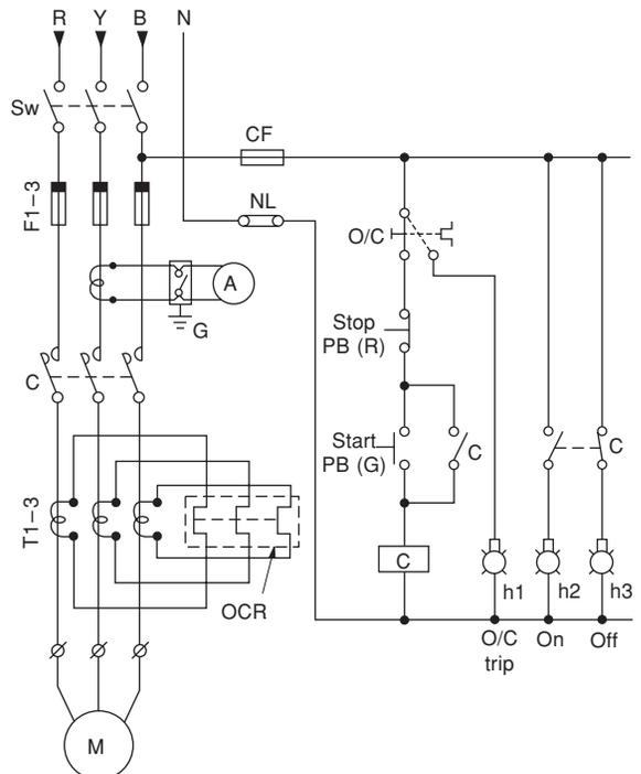
**Figure 13.54** DOL starter with CT-operated over-current relay
