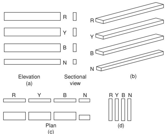
**Figure 13.30** Possible arrangements for busbar mounting systems
