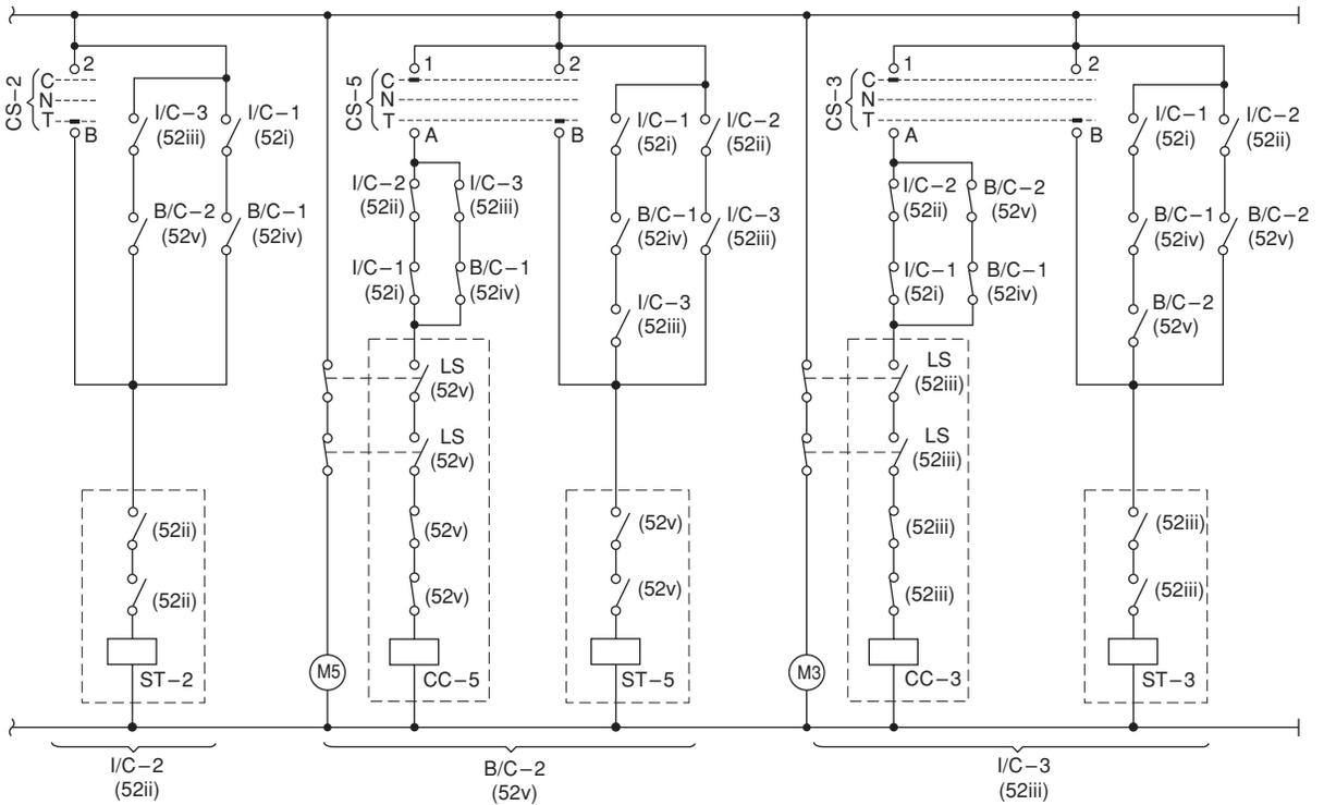
Figure 13.47 Control scheme for three electrically operated breakers, two bus couplers and three sources of supplies
