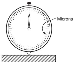
Figure A13.8 Thickness tester gauge
