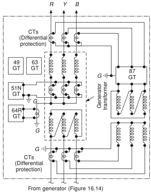
**Figure 13.47(b)** Protection scheme for a generator transformer (GT)
