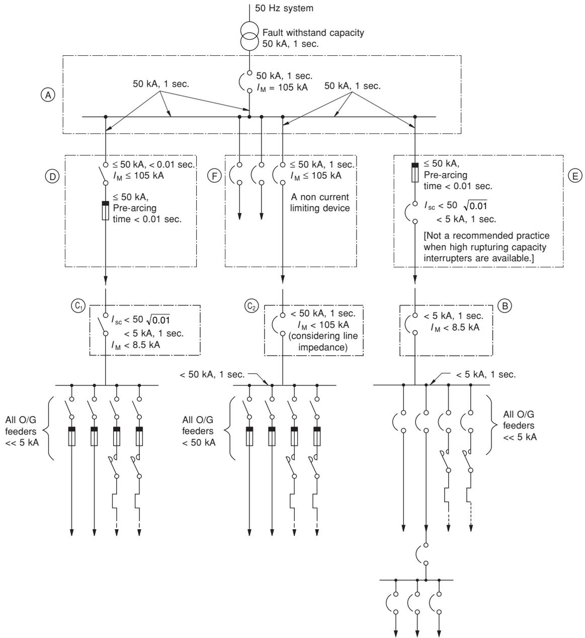
**Figure 13.29** An LV power distribution scheme illustrating the procedure to assign fault withstand capacity to a device, component or a bus system
