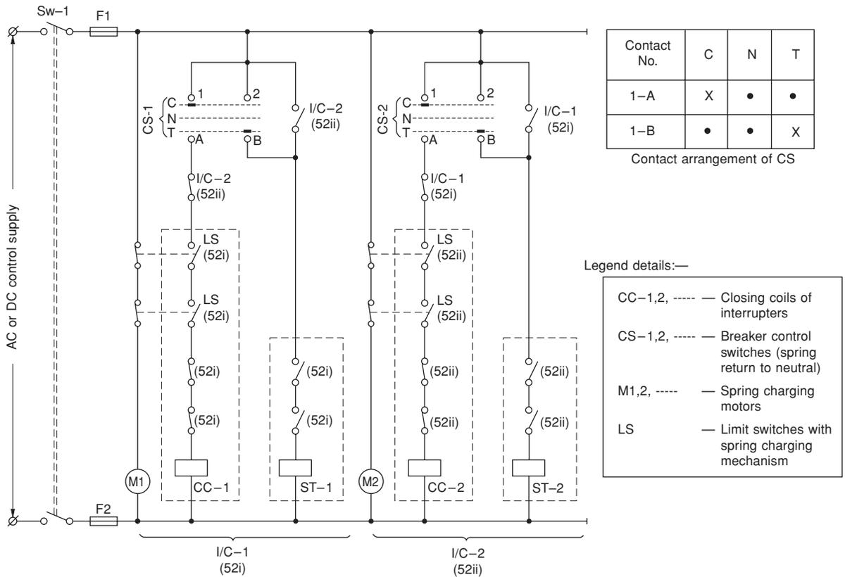
**Figure 13.45** Control scheme for two electrically operated breakers and two sources of supplies
