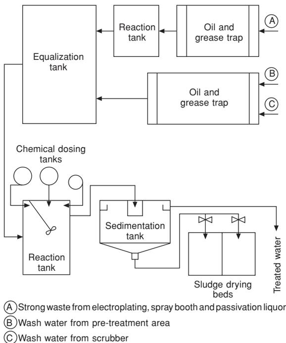
**Figure A13.11** Flow diagram – effluent-treatment plant
