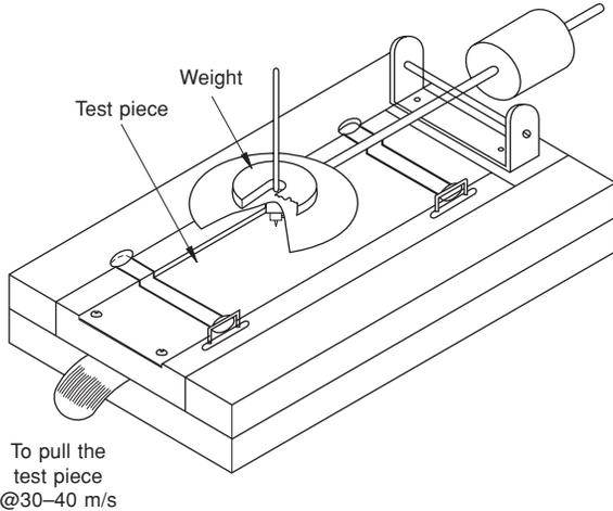
Figure A13.7 Scratch hardness testing apparatus
