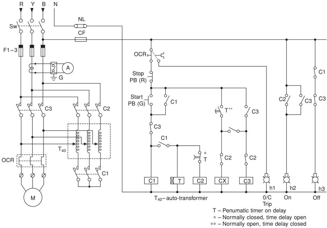
Figure 13.57(a) Auto-transformer starter using pneumatic timer
