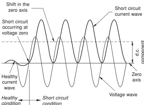
**Figure 13.26** Illustrating a shift of nearly 90° (drawn at 90° for ease of illustration) in the current wave at nearly 0.1 PF, fulfilling the condition of current lagging the voltage by nearly 90° yet rising together at zero voltage (minimum applied voltage)
