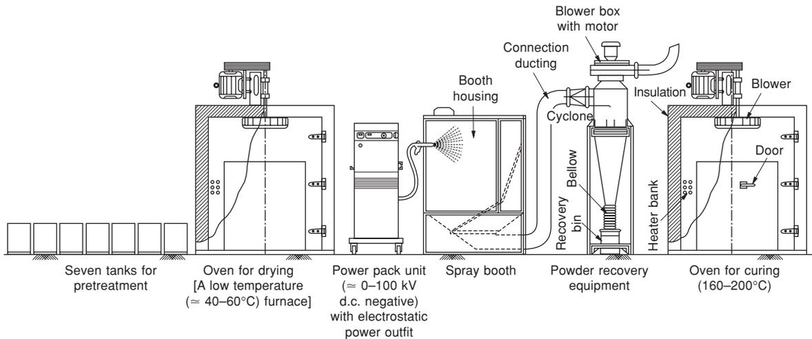
Figure A13.5 Single-line painting process for a powder system
