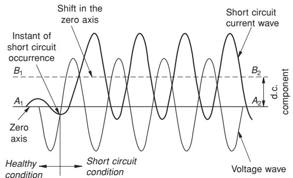
**Figure 13.27** Approximate illustration of a short-circuit condition occurring when both voltage and current waves are not at their natural zeros. Current shifting its zero axis from  $A_1$   $A_2$  to  $B_1$   $B_2$  to rise from zero again at the instant of short-circuit
