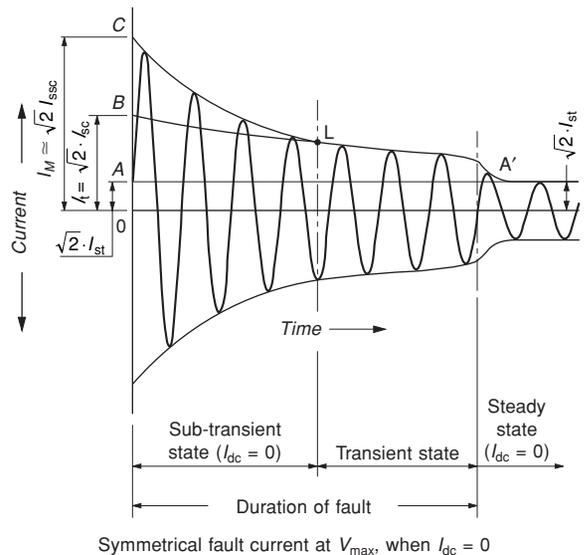
**Figure 13.19** Short-circuit oscillogram of a generator
