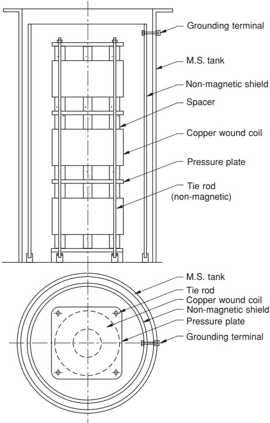
Figure 27.5 Sectional view of non-magnetically shielded reactor
