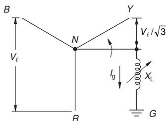
Figure 27.13 Neutral grounding reactor or a Petersen coil
