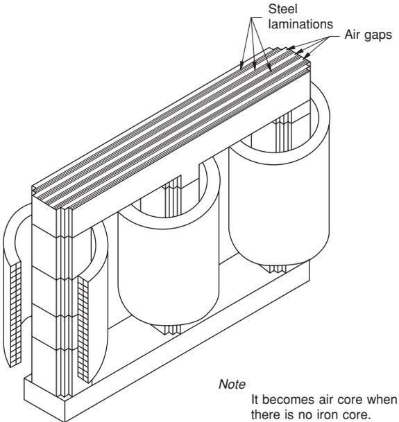
Figure 27.6 A gapped iron three-phase reactor
