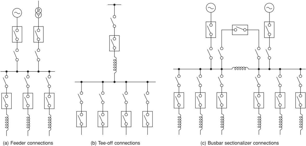
Figure 27.10 Series reactor connections
