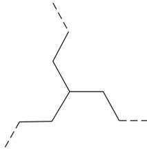
**Figure 27.7** Six- or nine-limb zig-zag arrangement of windings to limit the harmonics
