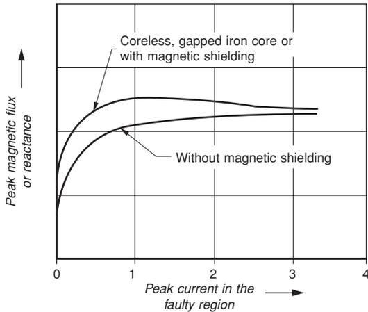
**Figure 27.11** Typical characteristics of a current limiting reactor (coreless, gapped iron core or magnetically shielded core type)
