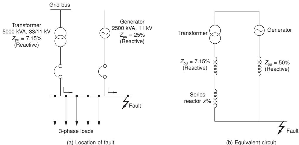
**Figure 27.12** Application of a series reactor
