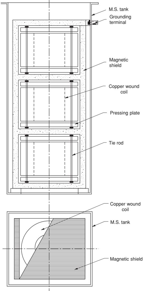
Figure 27.4 Sectional view of a magnetically shielded reactor
